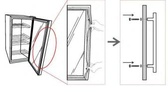
**Step 3** Insert the screw through the hole and connect with the handle.
