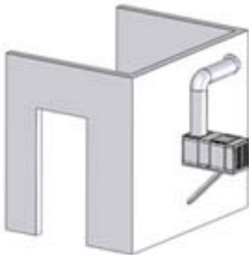
Through-Wall Inside Flush Mount
