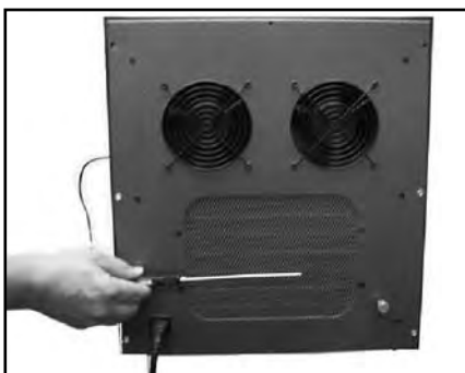
Inlet Air – Condenser (Back) Side•
